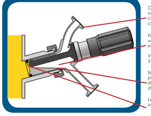
Choice of sanitary clamp or buttweld inlet and outlet connections. Custom connections also available
